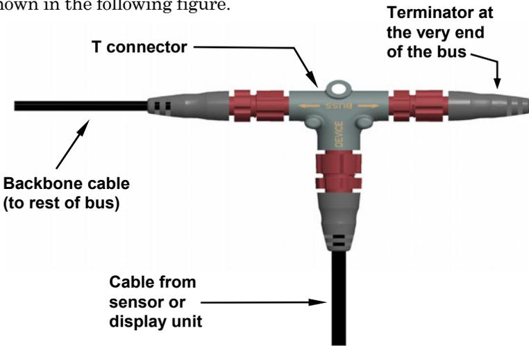
**NMEA 2000 network node located at the end of a NMEA 2000 bus.**
